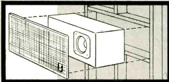
Custom-installation version of Wilton has snap-on grille that overlaps enclosure 1 1/2" on all four sides to cover gap between enclosure and wall framing or cabinet opening.
