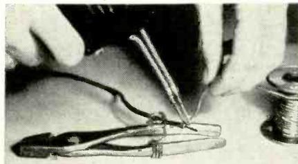
wrapped around a heavy tool such as a pair of pliers. Small parts can be held the same way. Try this "second-hand" idea sometime.—*Joe C. Allen*
