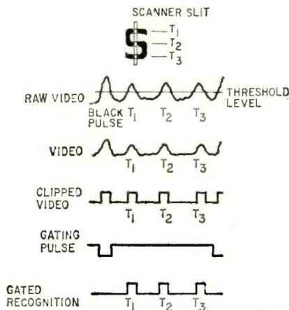
Fig. 4 — How recognition pulses are developed.
