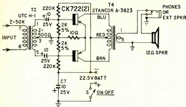
Fig. 2—Alternate power amplifier is used if greater power output is needed.
