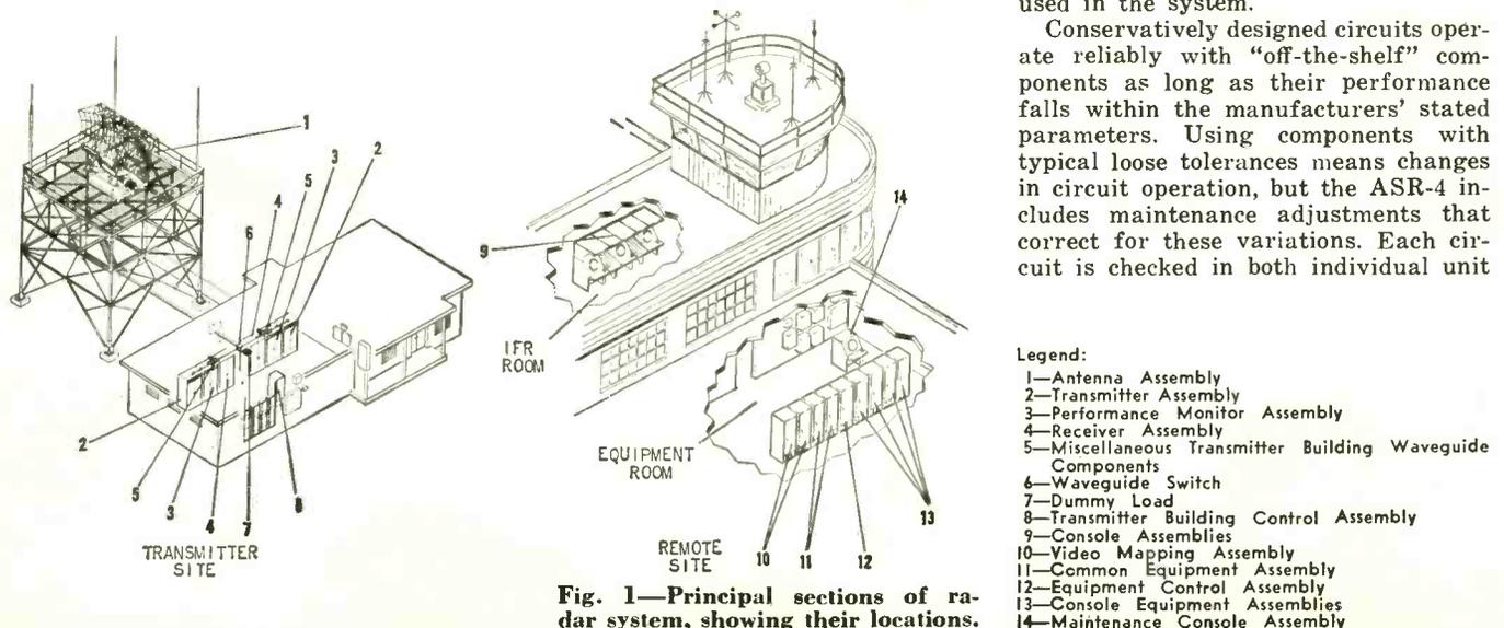
**Fig. 1—Principal sections of radar system, showing their locations.**
