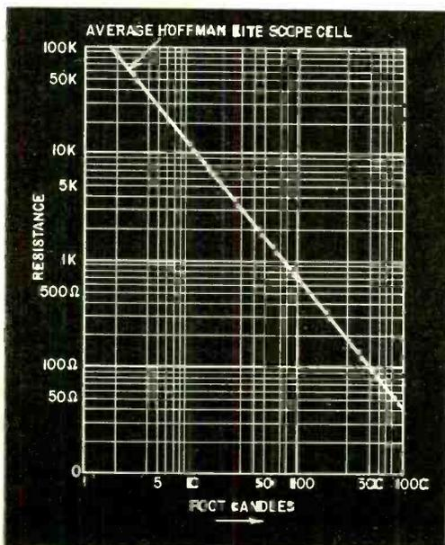
Fig. 2—Resistance of Hoffman photocell plotted against light intensity.
