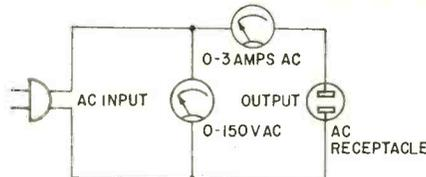
**Circuit of the instrument. Note that voltmeter is connected across input.**
