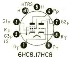
6.3 volts. The 17HC8 at 450 ma at 16.8 volts. The tubes are intended for use as vertical deflection oscillator and amplifier in TV receivers.
