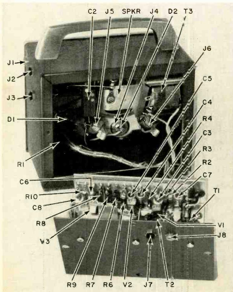
With its back removed, the parts layout inside the case is revealed.
