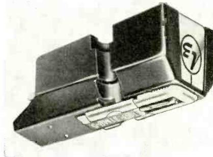
The stylus jewel is a diamond with a 0.5-mil radius. The compliance of the stylus is  $3.5 \times 10^{-6}$  cm/dyne in both lateral and vertical planes. The frequency response is rated at 20 to 20,000 cycles  $\pm 2$  db.
