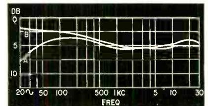
**Fig. 4**—Response of the recorder output: curve A, input to J1; curve B, input to J5.
