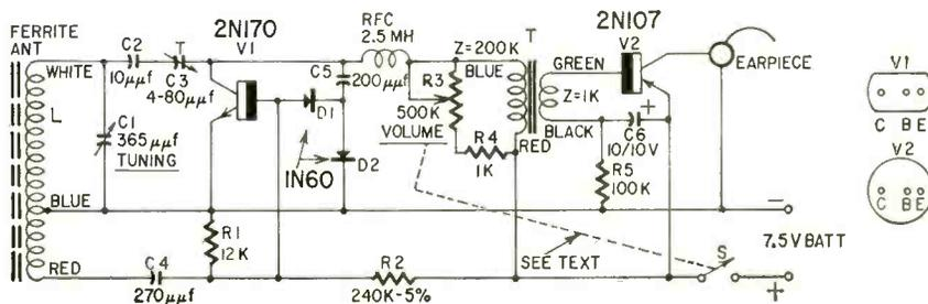
Circuit of the two-transistor receiver.
