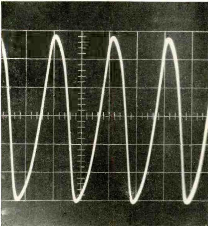
Photograph of oscilloscope tracing (using 5,000-cycle coil). Scope is connected across tuned circuit.
