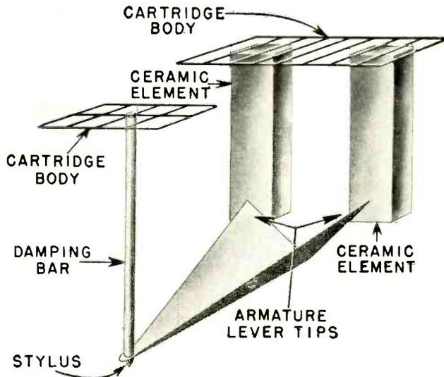
modulation of the stereo record groove is equivalent to a composite vertical and lateral signal, and each channel of the cartridge delivers an output voltage corresponding to the recorded amplitude of one of the channels of the stereo disc.
