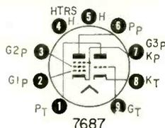
amplifier service while the triode is intended for use as a phase splitter. The 7687 features exceptionally low hum and noise. It is similar to the 7199 and is an improved low-noise version of that tube. Basing differs so the tubes are not directly interchangeable.
