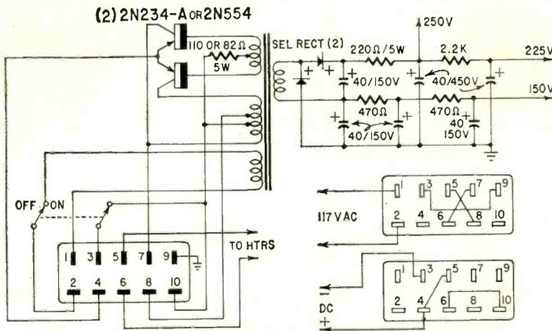
Fig. 5—Ac-dc power supply uses transistors.
