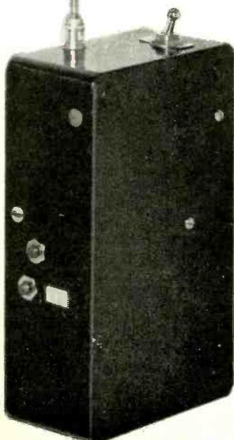
Upper button (S2) is for CW signal, lower button (S3) for AM signal.
