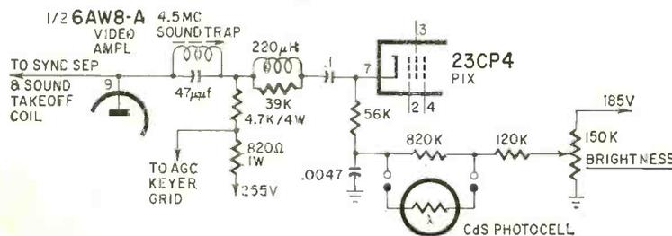
Fig. 1—Cathode circuit of the Lite Scope set.
