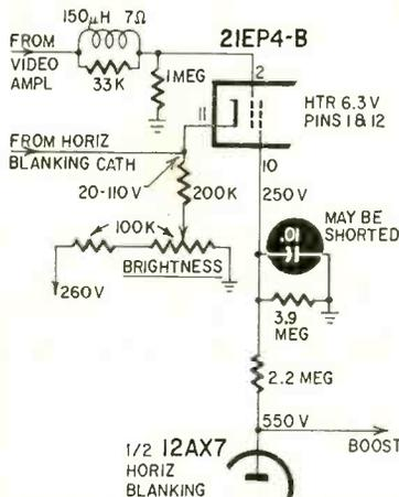
Fig. 4—Picture-tube socket connections in GE 21T7. If circled capacitor is shorted, no raster will appear.
