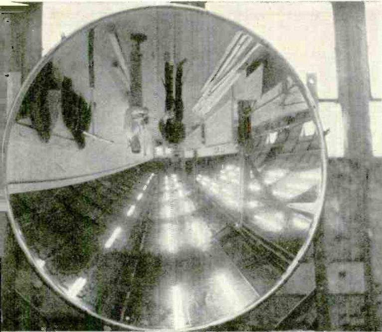
**UPSIDE-DOWN** image shows the near optical surface quality of this paraboloid radio mirror. Units are good uhf radiators (up to 100,000 mc). The 4-foot reflector shown was made by D. S. Kennedy & Co., Cohasset, Mass.
