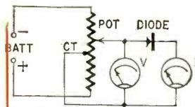
Fig. 1—Setup for plotting diode current as a function of voltage.
