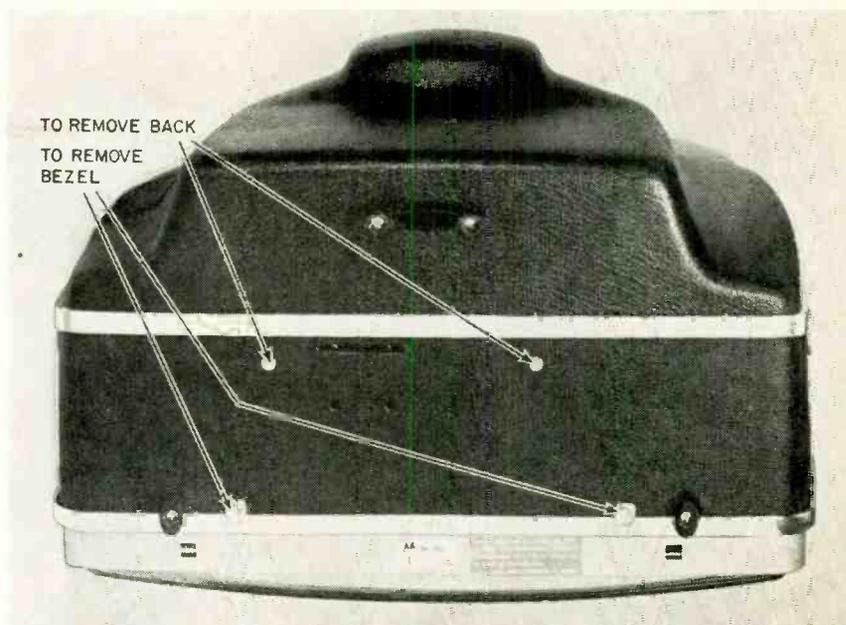
**Photo 3**—Bottom screws also hold bezel and back in place.
