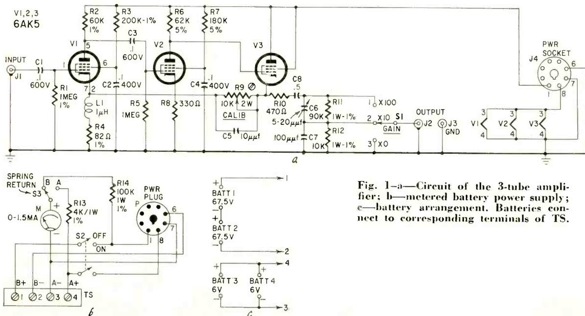
Fig. 1-a—Circuit of the 3-tube amplifier; b—metered battery power supply; c—battery arrangement. Batteries connect to corresponding terminals of TS.
