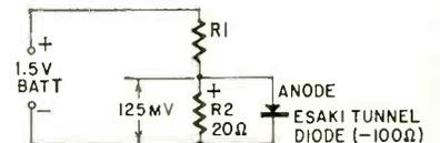
Fig. 5—Circuit for biasing tunnel diode from low source resistance.
