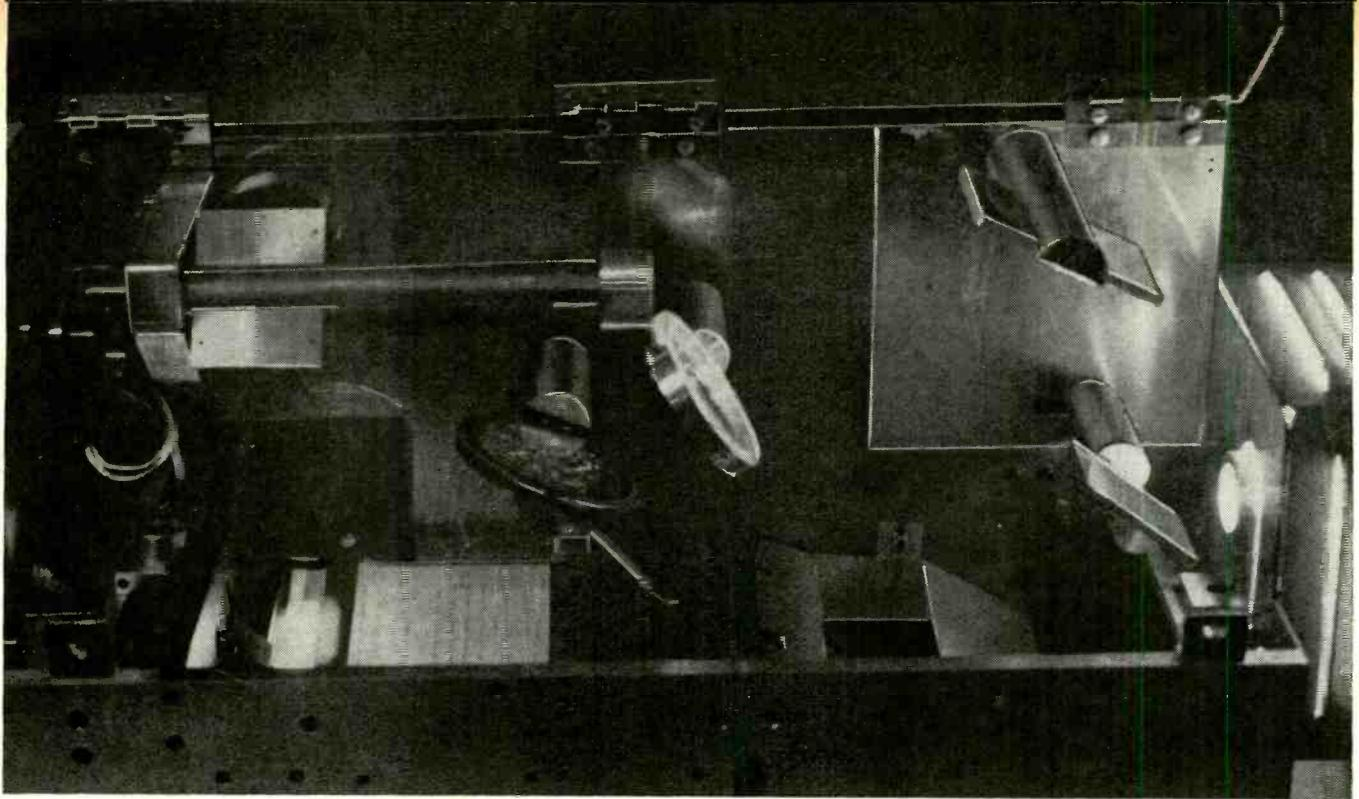
The "eye" of the Air Force print reader. It scans a message fed from the left. Light (at right) is transmitted through an optical projection system to the type-written page where it is picked up by the scanning device.
