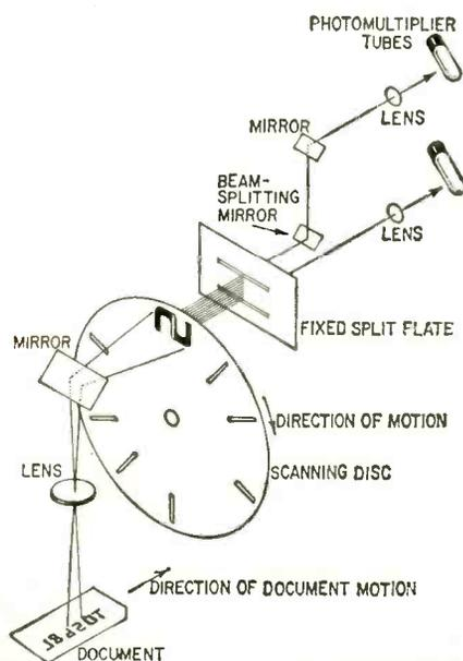
Fig. 1—The basic optical scanner.
