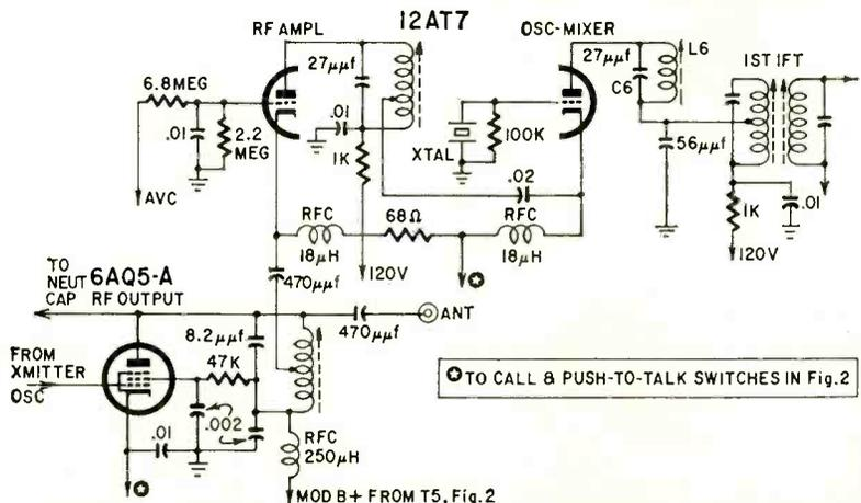
Fig. 3—Input and output stages of the Radson transceiver.
