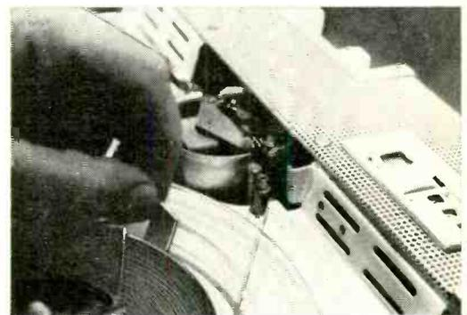
than to have recording tape spill when a reel is being handled. I keep this from happening by slipping a rubber band over the reel of tape as shown in the photograph. Even if the reel is acci-
