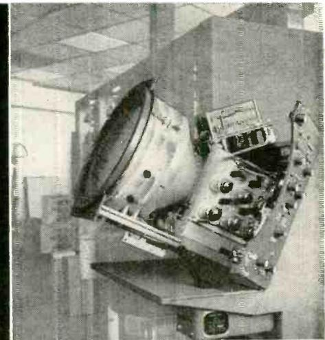
**(Left) How the equipment below the tube is rolled out.**
