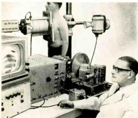
TV Fluoroscope combines doctor's fluoroscope with closed-circuit TV system. System reduces radiation exposure, increases clarity and detail. The TV picture can be recorded for reference. Dr. Russell H. Morgan of John Hopkins University described the arrangement at an American College of Radiology lecture.
