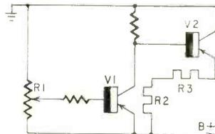
considerable current passes through heater coils R2 and R3. At higher ambient, V1's greater leakage current biases V2 to lower its conduction. Thus R1, R2 temperatures are lower to compensate for the higher ambient.
