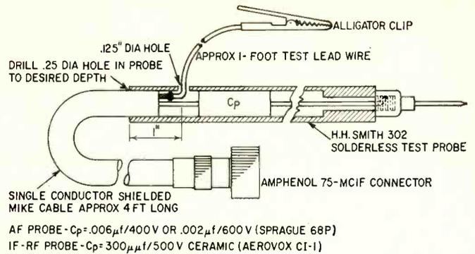
Fig. 3—Construction of the af and if-rf probes.
