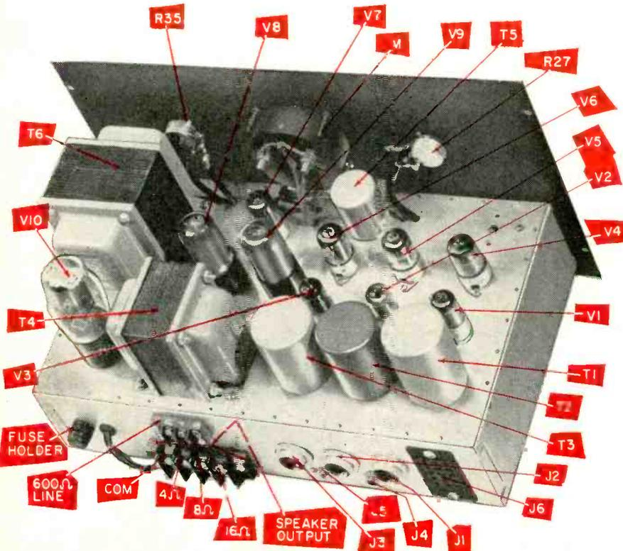
(Top) Front view of the amplifier showing the location of the controls. (Bottom) From the top, placement of all major components can be seen.
