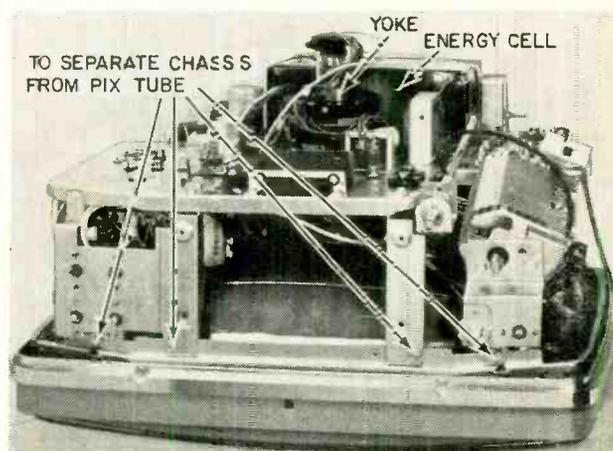
**Photo 4**—Four top screws hold chassis to picture tube. Two others are on bottom.
