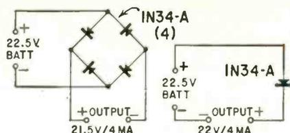
Fig. 5—Two protective circuits save components if battery is inserted incorrectly.
