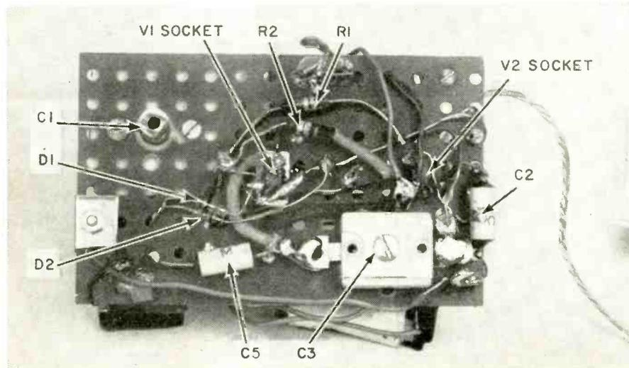
Some components are mounted on the wiring side of the chassis.
