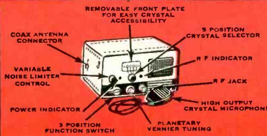
conversion to a push-to-talk relay a cinch. RF jack on the front panel may be used to monitor the current in the final tube using external meter.
