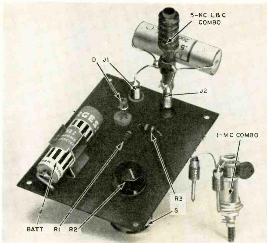
The tunnel-diode oscillator. The L-C combinations are attached to pin jacks for easy band changing.
