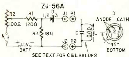
Fig. 7—Schematic of tunnel-diode oscillator. See text for values of L and C.
