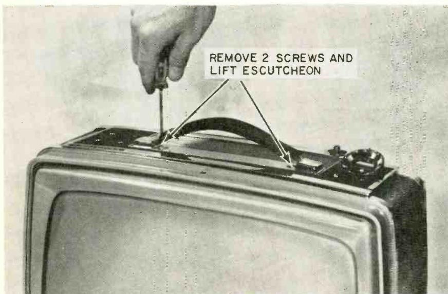
Photo 1 (Above)—First disassembly step is to remove knobs and carrying handle.
