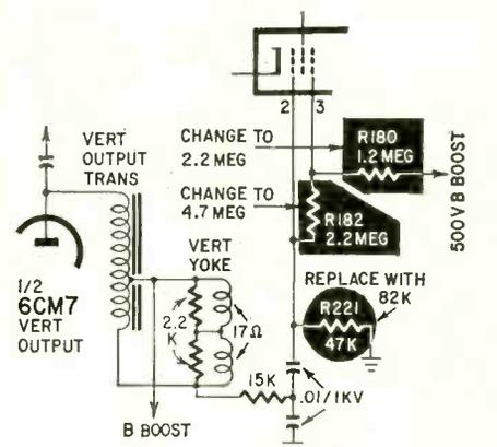
82,000-ohm resistor. As changing R221's value results in a dc voltage change in the circuit, resistors R182 must be changed from 2.2 to 4.7 megohms and R180 should be changed from 1.2 to 2.2 megohms.—Al Black
