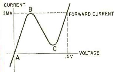
Fig. 3—Current-voltage characteristic of Esaki tunnel diode (GE No. ZJ-56A).
