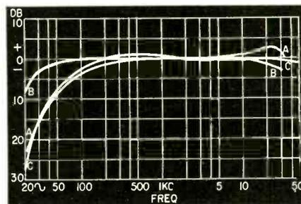
**Fig. 3**—Frequency response of the 600-ohm line output: curve A, input fed to J1; curve B, input fed to J5; curve C, line output with recorder input.
