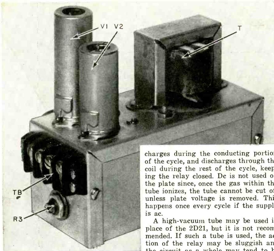
Top view. Relay contacts and grid of 2D21 connected to terminal board.
