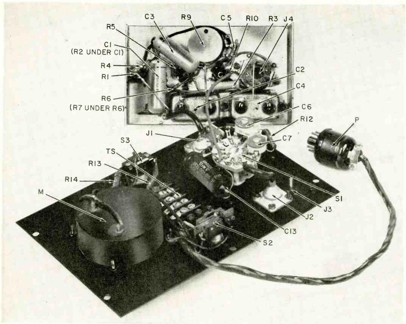
Disassembled unit shows construction details.
