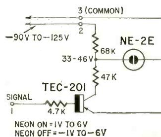
sulated body of the PCL (Printed Circuit Lamp). They connect to ground, B-voltage and a signal point. PCL's are made by Transistor Electronics of Minneapolis in 14 stock models to indicate a change in polarity at any desired low dc point in a circuit. In a typical PCL circuit, a change in polarity from anywhere between -1 to -6 volts to anywhere between 1 to 6 volts will turn the neon light on. Reverse signal polarity extinguishes the lamp. END
