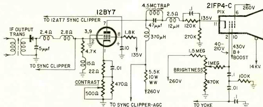
Fig. 3—Video-output circuit of Dumont RA-164, 165.
