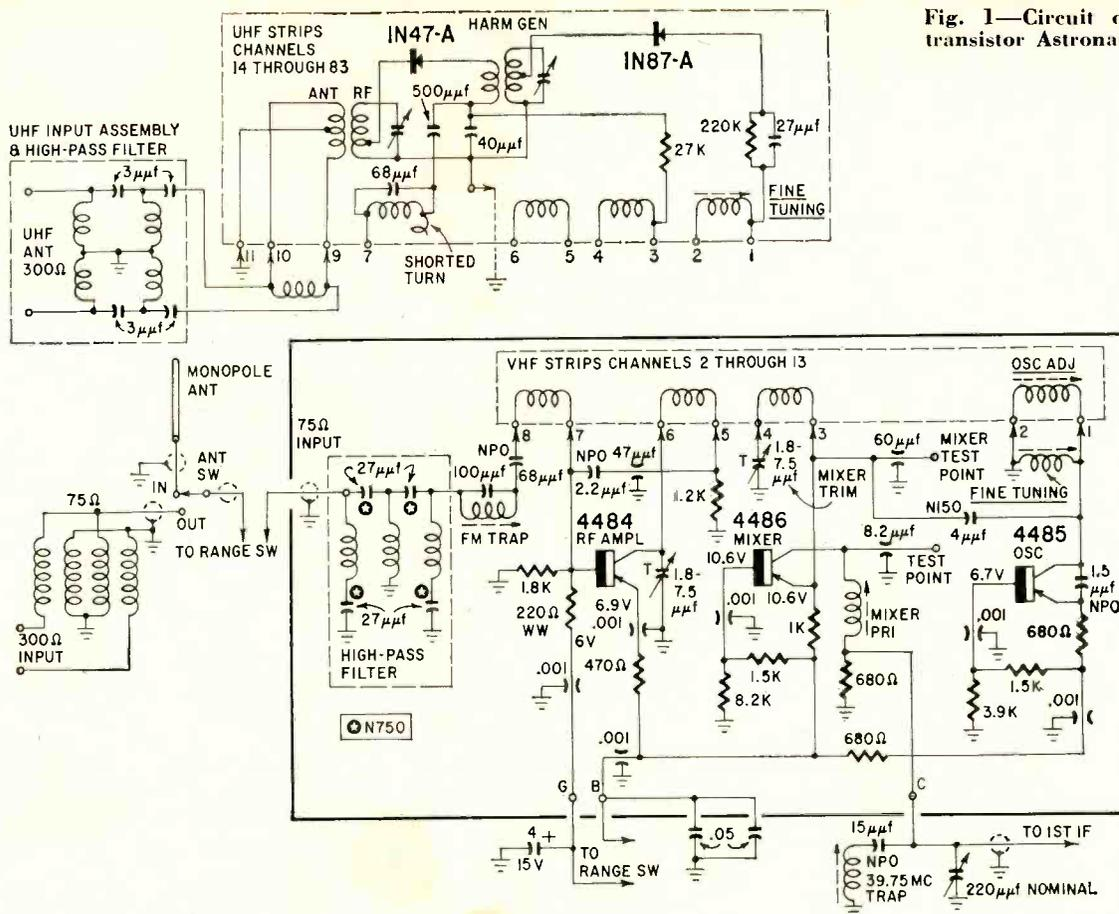
Fig. 1—Circuit of three-transistor Astronaut tuner.
