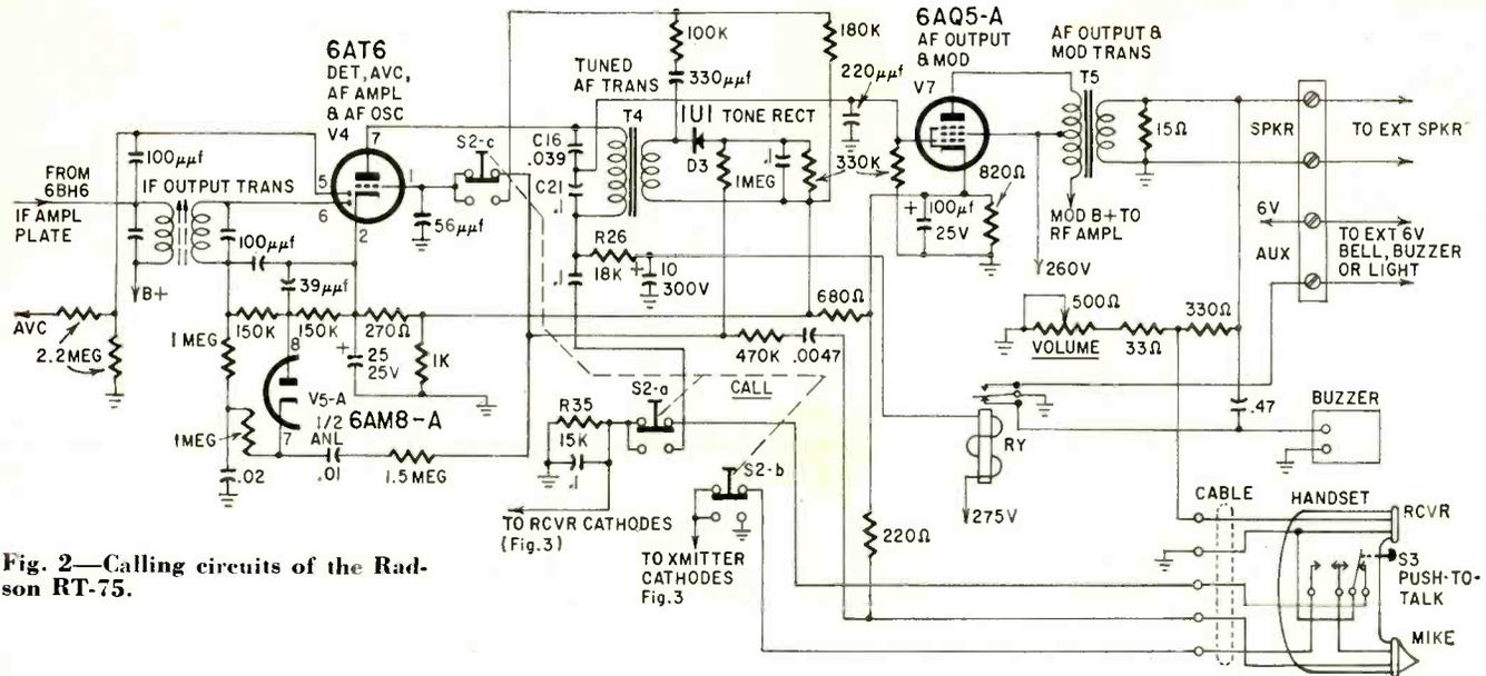
Fig. 2—Calling circuits of the Radson RT-75.
