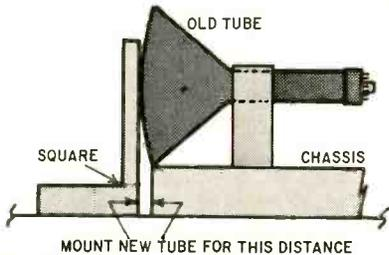
Fig. 2—Use a carpenter's square to measure the distance between the chassis apron and the picture-tube face.
