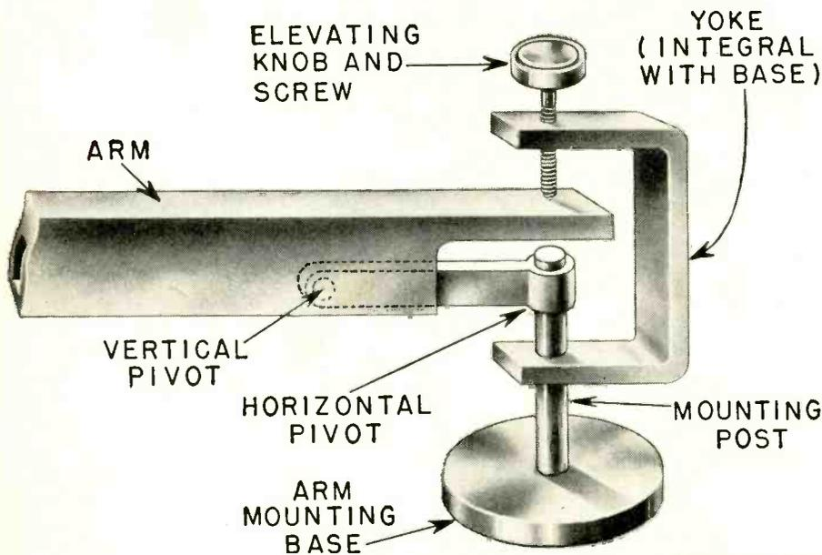
Fig. 4—Elevating screw allows the CS-1 to be raised and lowered without changing the lateral position of the stylus.
