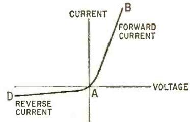
Fig. 2—Current-voltage characteristic of a typical p-n junction diode.
