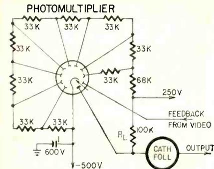
Fig. 3 — Circuit of photomultiplier in scanning device.
