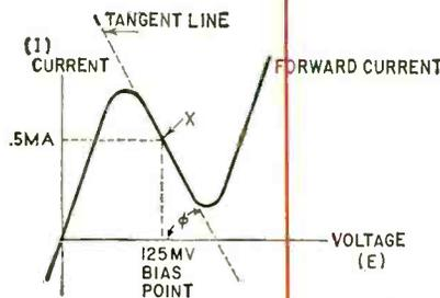
Fig. 4—Slope of characteristic around point X indicates negative resistance.
