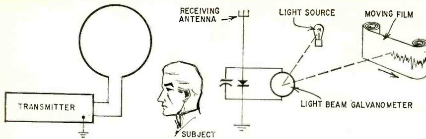
Fig. 1—Cazzamalli used this simple set-up to detect "radiation" from human subjects.
