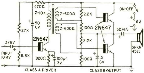
class-B output stage. This arrangement needs no output transformer and the
