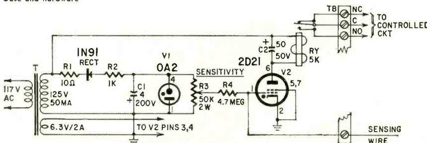
Schematic of proximity relay. Spst on-off switch may be added.
