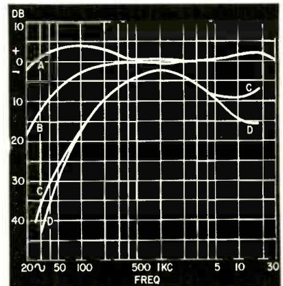
Fig. 1—Frequency response curves with signal input to J1. Output taken from the 16-ohm speaker terminals: Curve A shows response with bass and treble controls set at maximum with the bass boost circuit operating. Curve B is the same as curve A, except that the bass boost circuit is switched out. In curve C, tone controls are set at half scale, and in curve D, in minimum position.
